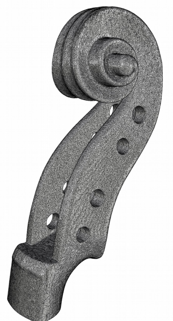
Figure 6: triangle mesh, perspective view of the scroll of the violin of figure 1
