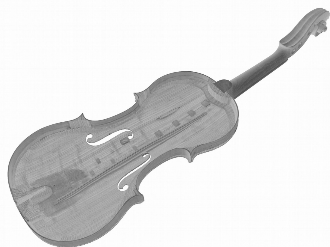
Figure 2: perspective view of the 3D rendering of Figure 3, showing the interior of the violin, with the back plate removed
