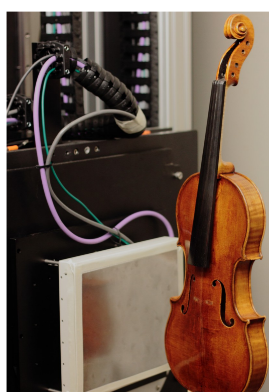
Figure 1: experimental set-up, with the flat panel detector on the left of the violin
